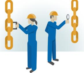
Magnetic Particle Inspection of each link. Visual control of shape, studs and surface of each link.
