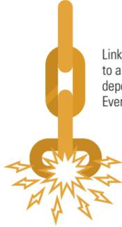
Links are flash butt welded according to a specific welding recipe that depends on chain grade and size. Every flash weld is recorded.
