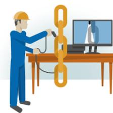
Phased Array method uses ultrasonic waves with a large number of scanning beams to check the interior of the welded area on the link. The versatility and high speed of the PA method enables 100% check of all welds.
